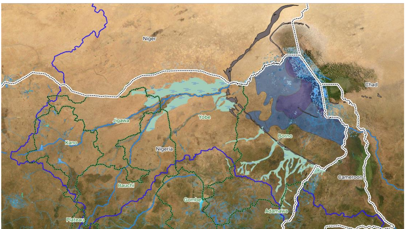
Figure 6: Alluvial floodplain deposits associated with the contemporary Bama Ridge Sand Barrier. Also shown shaded in blue tones are the Middle Chad high yield artesian aquifer (a1) and moderate yield artesian (b1) and moderate yield sub-artesian (b2) aquifers. The Middle Chad trends parallel the modern shoreline and tributary trends.
