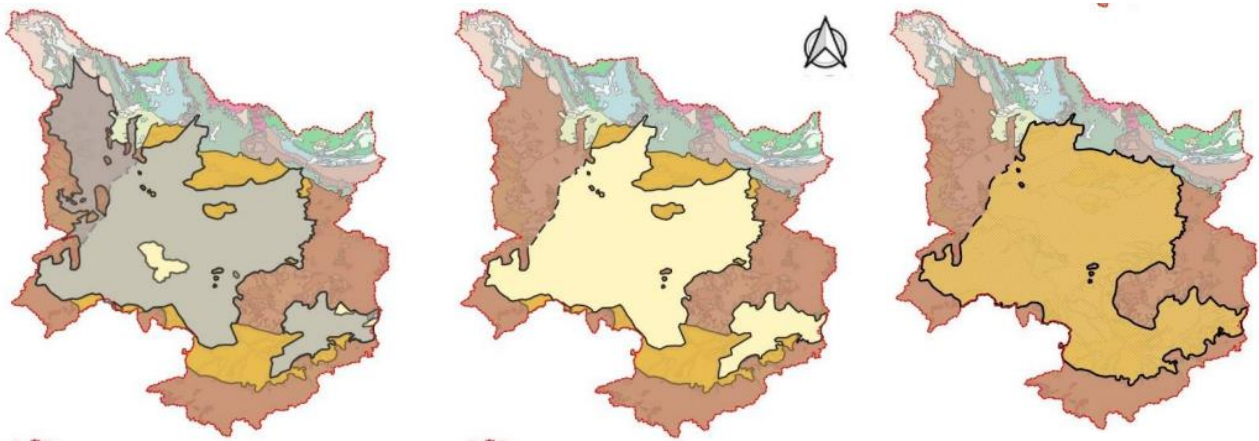
Figure 8: Spatial extent of major geological formations represented in CIWA 2020 numerical groundwater model for the Lake Chad Basin. Gray: Quaternary; pale yellow: Upper Pliocene Clay; orange: CT ± Middle Chad Formation; brown: Bedrock (including Cretaceous Basins & Pre Cambrian Basement).
